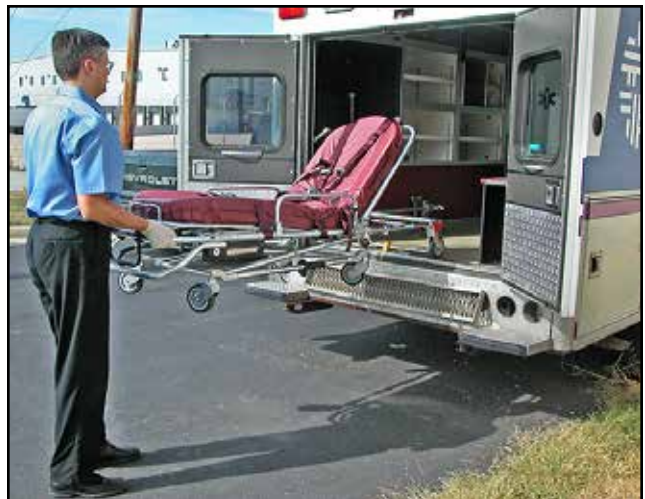
Figure 31 - Cot Level With Ambulance Floor
