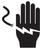
Ensure power source matches voltage identified on appliance rating tag. The rating tag provides essential technical information required for any appliance installation, maintenance or repairs. Do not remove, damage or modify the rating tag.
