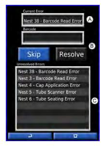
**A**: This box displays the current error being dealt with. You must perform some action on each error.
