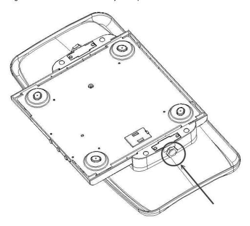
**4.** Scale assembly is finished. Turn scale over to begin weighing operations.
