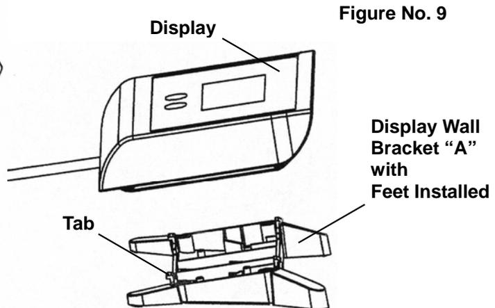
4. Referring to Figure No. 9, align and insert the tabs on the bracket with the slots in the display back and press together until the bracket locks to the back of the display.
