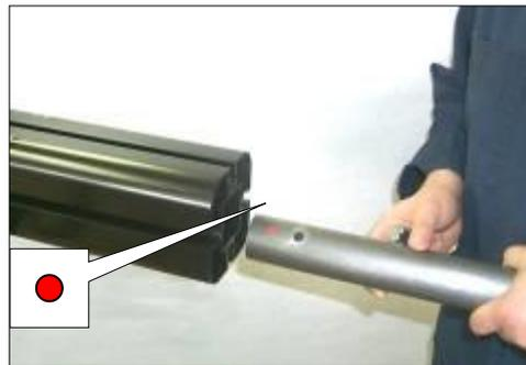
**Step 2:** Install washer (C-003293) onto the end of the bar.
