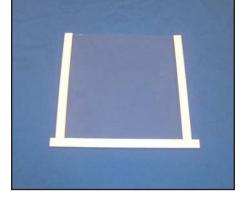
Using the four clamps supplied, clamp each of the four outside corners of the gel sandwich assembly. If desired, using the bottom spacer is not required. Simply, align side spacers with bottom of glass plates and tape bottom edge of glass plate assembly with casting tape (CTP-125). When taping bottom of glass plate assembly make sure to fold tape up around the corners approximately 1 inch.
