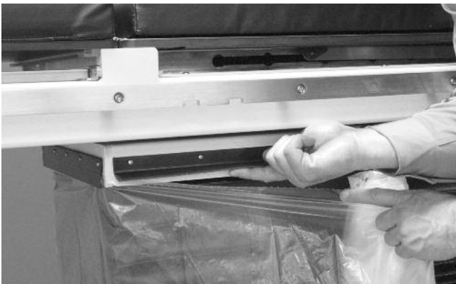
Figure 6. Lift the lower section of the strip on each side of the table, slide the plastic skirt underneath and lower the strip to hold the skirt in place.
