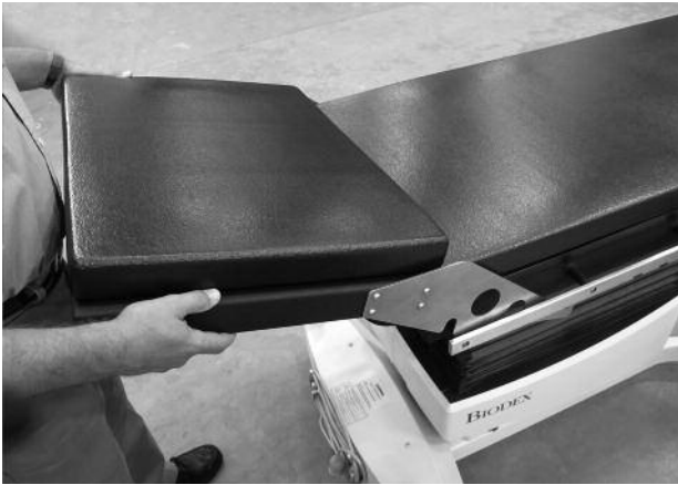
Figure 4. Installing tabletop extensions.
