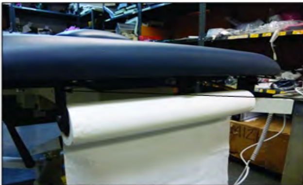
Figure 10. Using a 7/16" wrench, install the two 1/4-20" hex head screws removed in step 1 through the dispenser mounting bracket and tighten to secure the paper dispenser bracket in place. Repeat steps 1 - 4 for the opposite side.
