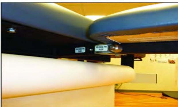
*Figure 13.* Place a roll of paper on the paper dispenser rod and install the rod between the brackets. Press in on either spring-loaded end of the paper dispenser bar in order to slide it into the brackets.
