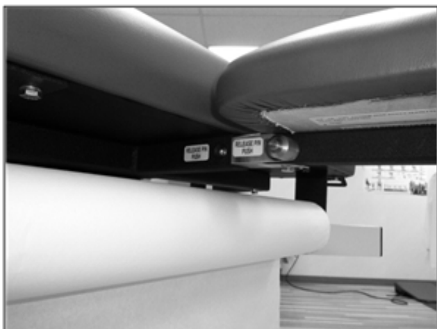
Figure 12. Place a roll of paper on the paper dispenser rod and install the rod between the brackets. Press in on either spring-loaded end of the paper dispenser bar in order to slide it into the brackets.
