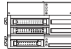
Incorrect Mounting Direction
