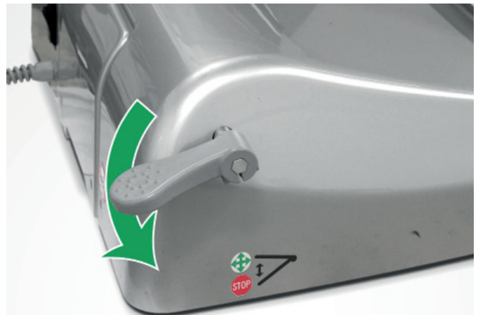
Fig. 23 Locking the casters
