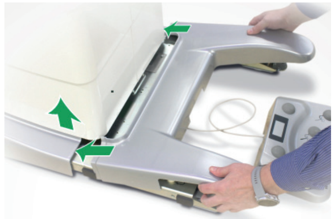
Fig. 13 Placing the front foot cladding
