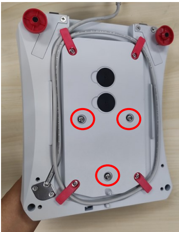
a) 3 screws installation method
