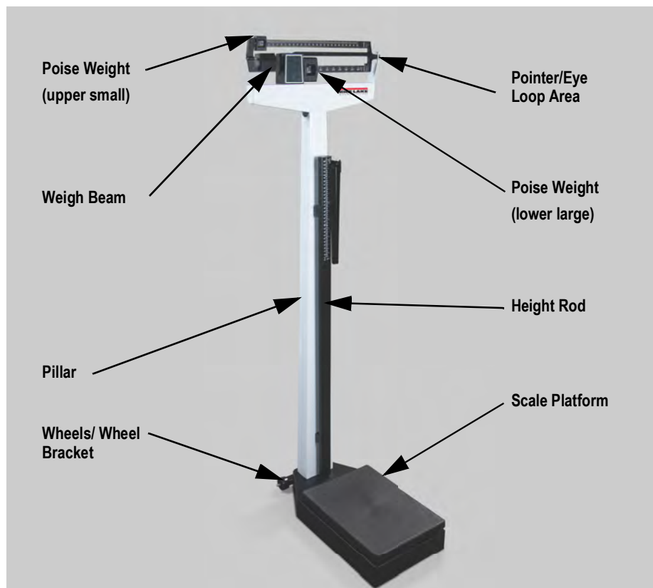
Figure 2-1. RL-MPS-50 Parts
