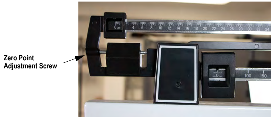
Figure 3-1. Poise Weights Set to Zero
