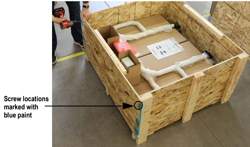
Figure 2-3. Side Panel Screw Removal
