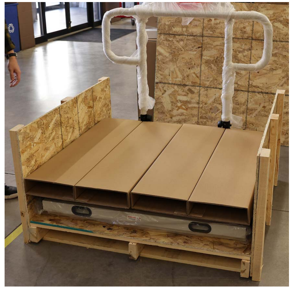
Figure 2-5. Raising Handrail and Removing Cardboard Platforms
