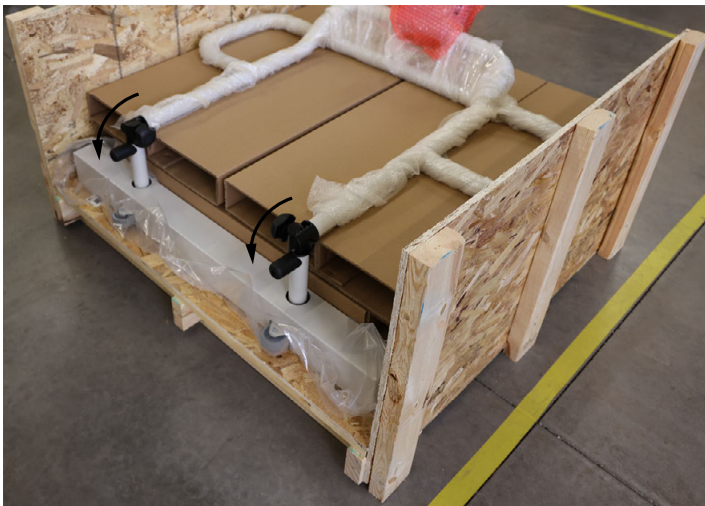
Figure 2-5. Raising Handrail and Removing Cardboard Platforms
