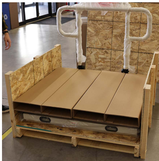
Figure 2-5. Raising Handrail and Removing Cardboard Platforms
