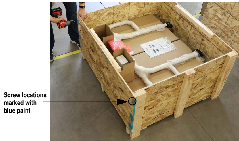
Figure 2-3. Side Panel Screw Removal
