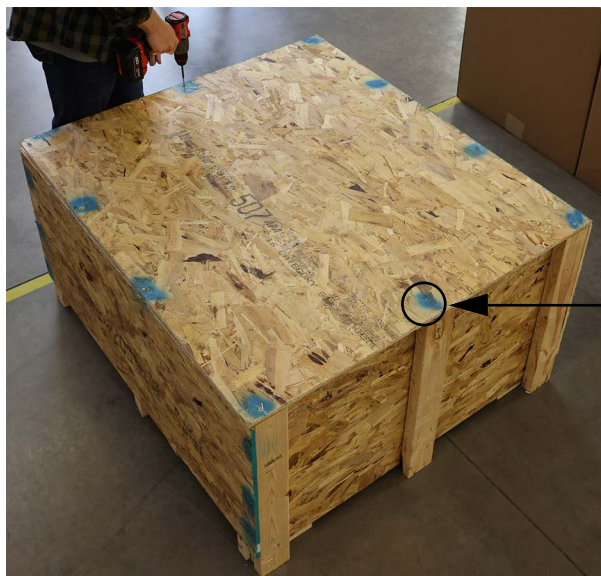
Figure 2-1. Crate Cover Screw Removal
