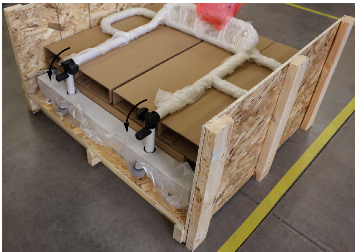
Figure 2-5. Raising Handrail and Removing Cardboard Platforms
