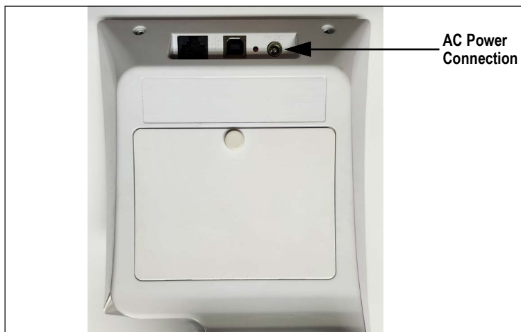
Figure 2-8. Power Connection Site
