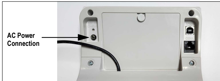
Figure 2-2. Power Connection Site
