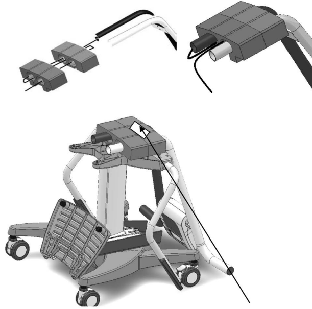
Figure 2-7. Remove Styrofoam Packing Pieces From Main Handle
