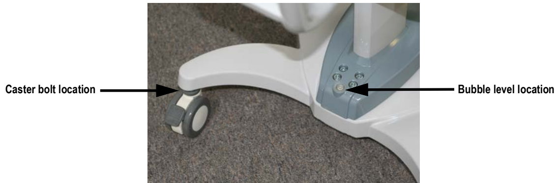
Figure 2-14. Bubble Indicates That The Scale is Level
