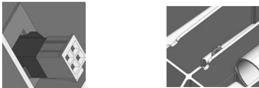
Figure 2-10. Connect Load Cell Cable and Indicator Cable
