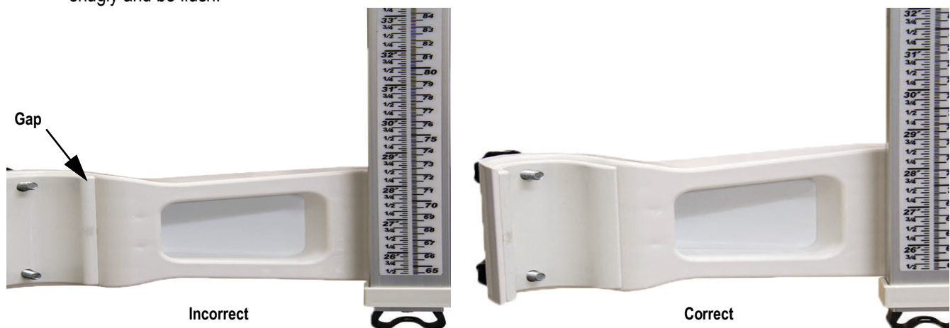
Figure 6-2. Bracket Insert Placement
