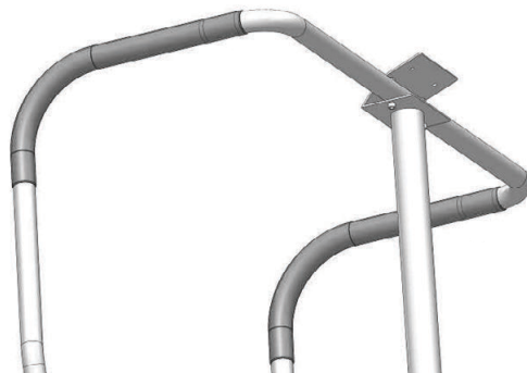
Figure 2-6. Rubber Grips in Proper Position
