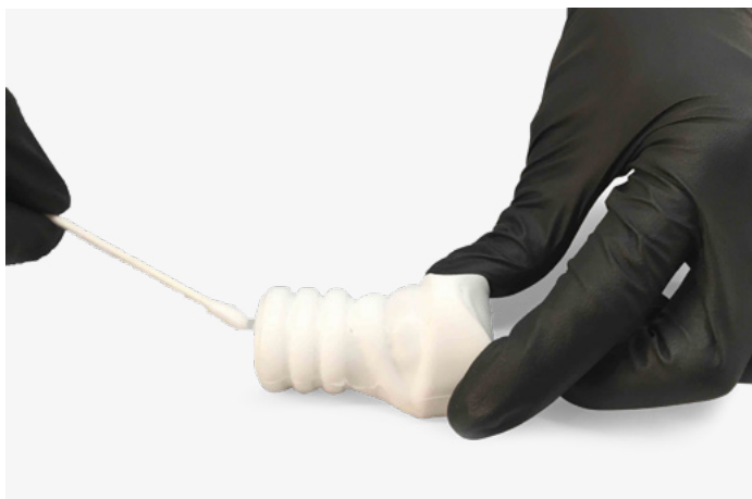
5. Using a cotton swab, enter the trachea from the inferior aspect and wipe away any excess silicone that may be on the inside of the trachea.
