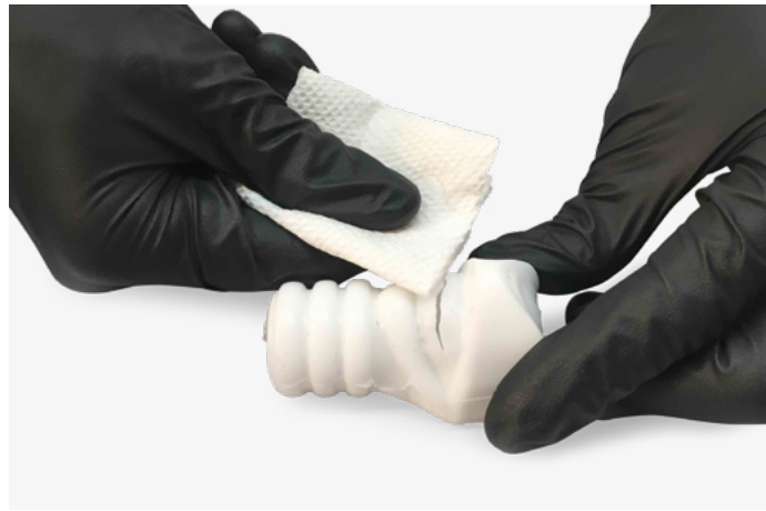
2. Clean site with 99% alcohol and cloth, wiping away excessive dirt and debris. (Note, any dirt or debris left on repair site will be permanently sealed into the repair.)
