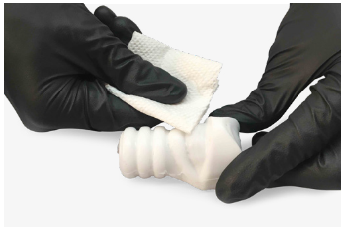
6. Wipe repair site with 99% alcohol to remove excess silicone.
