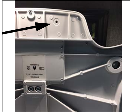
Figure 3-1. Setup Switch Location
