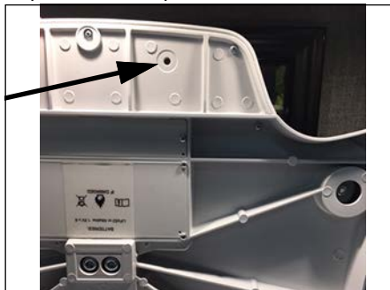
Figure 4-1. Setup Switch Location
