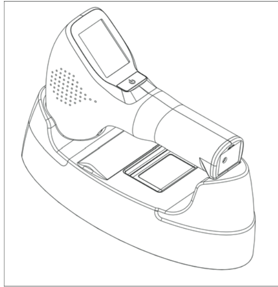
Figure 4-3 M1-W/M1 Place the Instrument on the Docking Station
