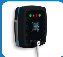
EL-IOT-1 WiFi Ambient temperature data logger
