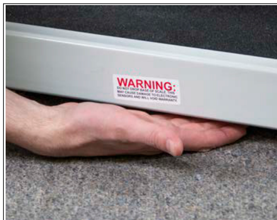
Figure 2-5. Scale Base Clearance
