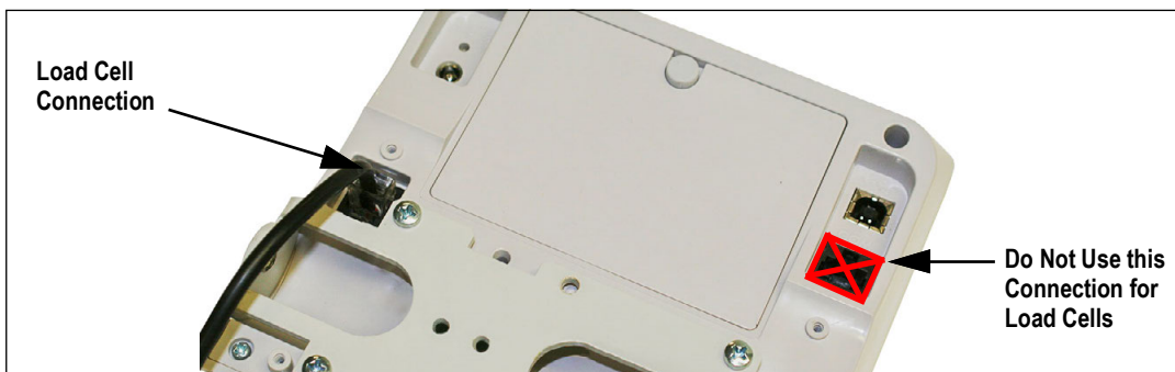
Figure 2-12. Load Cell Connection Point
