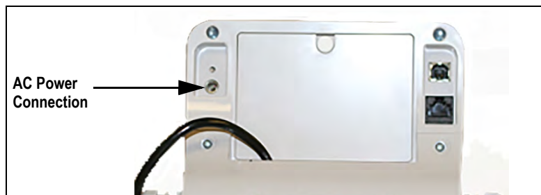
Figure 2-5. Power Connection Site
