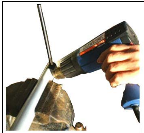
Figure 2. Heat the Damaged Hinge
