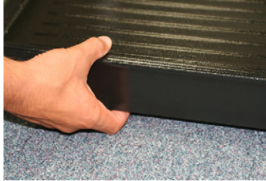
Figure 2-2. Clearance Between Scale Base and Floor
