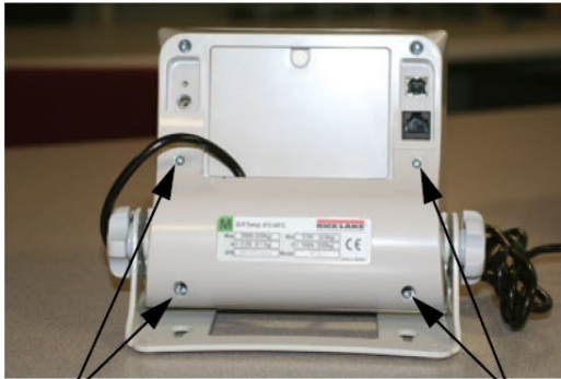
Remove four screws to access setup switch
