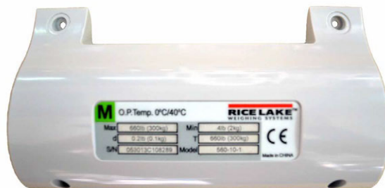
Figure 2-10. Attach Molded Back Cover onto Indicator
