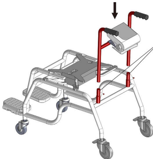
Figure 2-5. Insert Handle Assembly to Chair Frame
