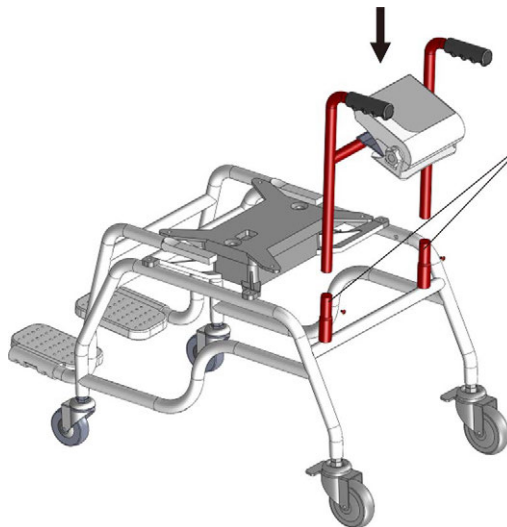
Figure 2-5. Insert Handle Assembly to Chair Frame
