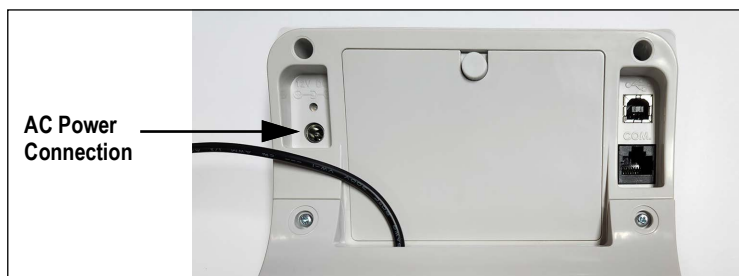
Figure 2-11. Power Connection Site
