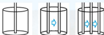
Multiple aspiration point settings (one, two or three positions) to optimize liquid aspiration from different plate types
