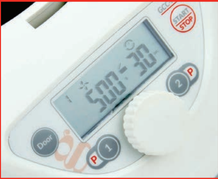
Two program buttons enable simple programming and recall of regularly used methods
