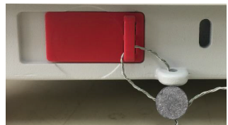
Locked with Wire Seal
