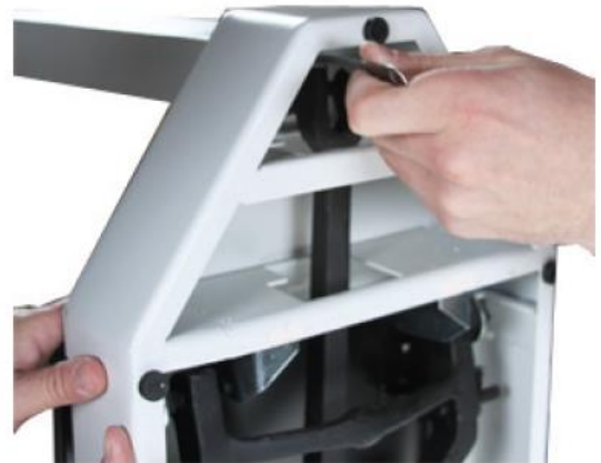
Figure 2-4. Connecting the Steelyard Rod to the Scale Base
