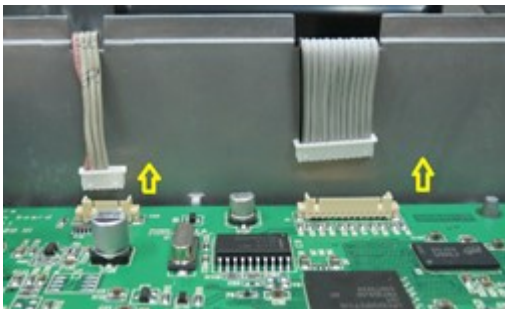
Figure 2-24 Load Cell Cable Connecting to Main PCBA Removed.
