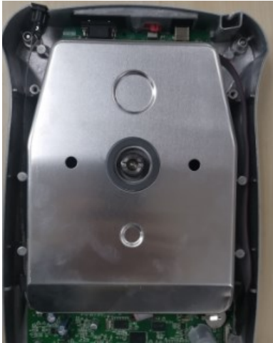
Load cell metal cover attached
