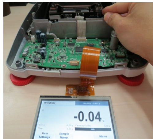
Figure 3-62. Adjust position of Sensor Board until Over load does not appear.
