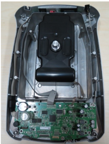
Figure 3-27 Adventurer Analytical Load cell metal cover removed.
