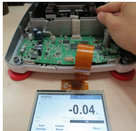
Figure 3-75. When Position Sensor Board shows normal weight, tighten its screws with an Allen Key.
