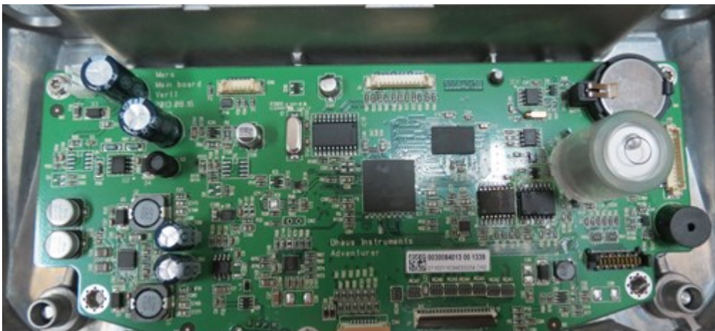
Figure 3-38 Two cables removed from main PCBA.
