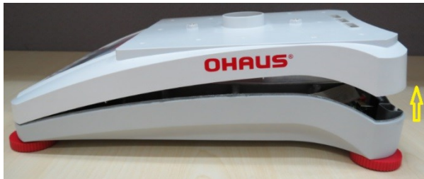
Figure 3-9 Lifting up the back of Adventure top housing.
