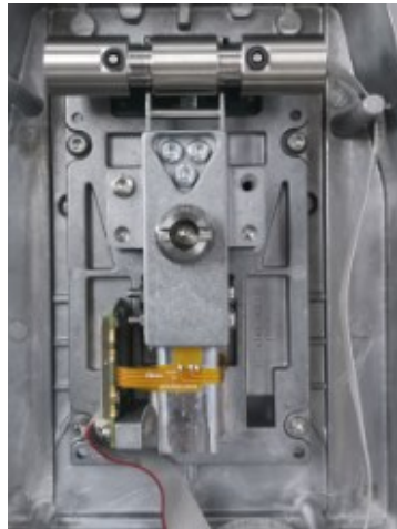
Load cell metal cover removed
