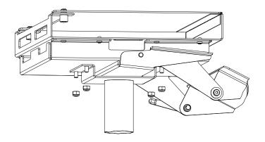
Place the Housing/Keyboard Tray Assembly onto the Upper Column Assembly. Thread the nuts onto the mounting a 7/16' wrench
