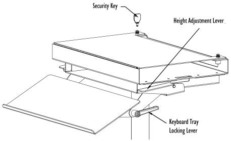
To open the cover and insert your computer, use the Security Key to turn the fasteners 1/4 turn counter-clockwise. The fastener should pop up to give a visible indication that it is unlocked. To refasten, use the key to push the fastener back into it's socket and turn clockwise until locked.
