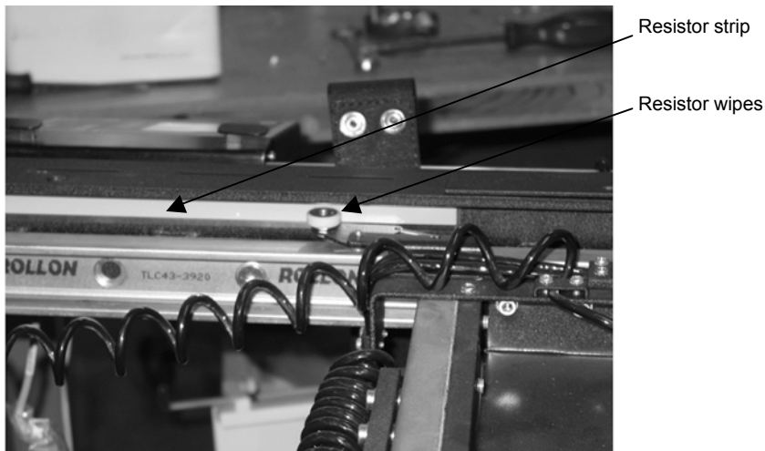
Figure 10.4. X position sensing resistor strip (tabletop removed for viewing.)
