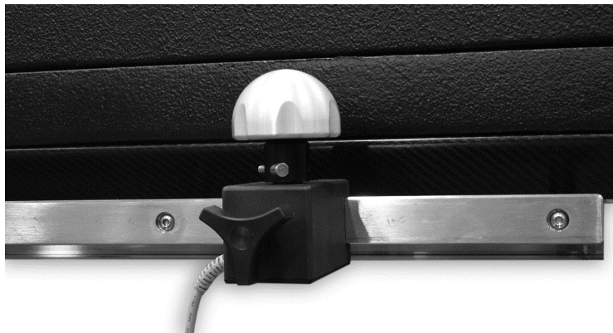
Figure 2.5. Push button (on handle) releases tabletop for free-float X-Y motion.
