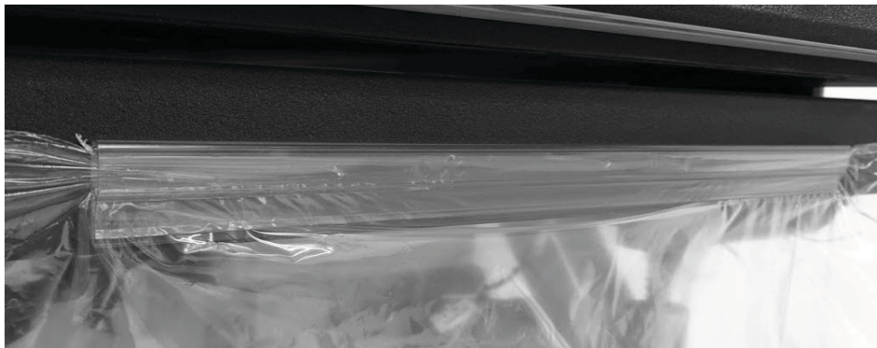
Figure 2.7. Slide the plastic skirt underneath and lower the clip to hold the skirt in place.
