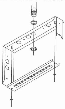
WHEN INSTALLING DIRECTLY TO CONDUIT FROM THE TOP OF THE UNIT REMOVE LED ASSEMBLY. THREAD CONDUIT NUT ONTO FITTING BEFORE INSERTING INTO KNOCKOUT HOLE. SECURE FITTING TO UNIT WITH SECOND CONDUIT NUT LEAVING MINIMUM FITTING THREADS IN THE ENCLOSURE FOR THE LED LAMP ASSEMBLY TO BE REMOUNTED OVER.
