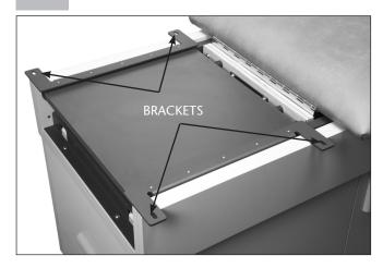
Secure the seat to the seat brackets using (4) four 1" hex head bolts and 1/4" washers.
