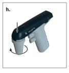
**h.** Press the upper housing section into the housing shells and screw on the adapter housing.
