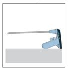
The accu-jet® S can be set down on an even surface with an inserted pipette.
