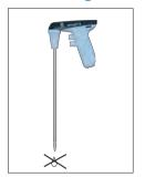
After adjusting the meniscus, no liquid should drip from the pipette without operating the valves. If the pipette is dripping, see Troubleshooting, p. 51
