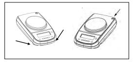
It is important to allow the balance to equilibrate to the ambient environment after powering on, and before using. For 0.0001g balances, allow the balance to equilibrate for 2 hours. For 0.01mg balances, allow the balance to equilibrate for 12 hours. For calibration procedures, please refer to the "Device calibration chapter". Perform the device calibration whenever it is moved to another place.
