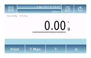
In the weighing screen, the area displaying the weight shows the value of the weight on the weighting plate.
