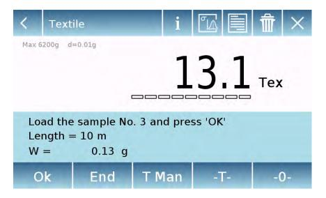
Tap the **"Ok"** key to acquire a new weight. Tap the **"T Man"** key to enter a manual tare value Tap the **"-T-"** key to run a manual tare Touch the **"- 0 -"** key to reset the plate.
