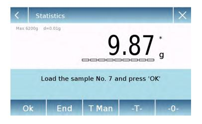
Tap the " **Ok**" key to capture a new weight. Tap the " **T Man**" key to enter a manual tare value Tap the "-**T**-" key to run a manual tare
