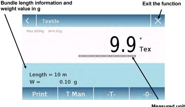
Tap the "**Print**" key to print the result. Tap the "**T Man**" key to enter a manual tare value Tap the "**-T**-" key to run a manual tare Touch the "**- 0** -" key to reset the plate. Measured unit selection key displayed
