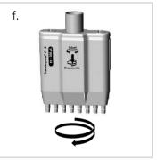
f. Reassemble the pipetting unit. The pipetting unit must be screwed onto the hand grip in a counter-clockwise direction until it clicks into place. Check the instrument for leaks, see p. 52.
