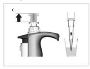
Allow the pipetting button to steadily move back to its original position.
