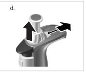
d. Slide the red adjustment slider back completely, lift the volume-setting wheel (decoupling) and release the adjustment slider.
