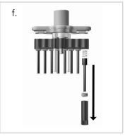
f. Remove the piston nut and pull off the piston with piston spring.
