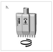
h. Reassemble the pipetting unit. The pipetting unit must be screwed onto the hand grip in a counter-clockwise direction until it clicks into place. Check the instrument for leaks, see p. 52.
