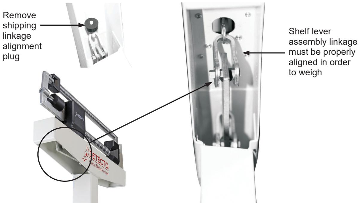
**Figure 6. - View of linkage underneath weigh beam headpiece**
