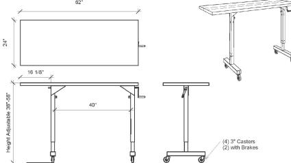
Designed to adjust to the height of the patient table during CRT implantation & extraction. Extension allows for RAO camera rotation without hitting the legs of the table.
