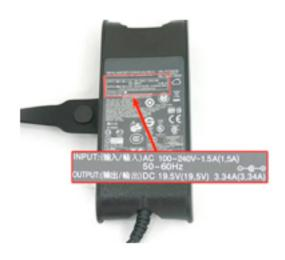
After charging your battery, check the back of your device's charger to determine the proper output voltage. If the output is 18-20 Volts the switch should be left in the default 19 Volt position. If the output is 11-13 Volts, use a sharp pencil to move the switch to the 12 Volt position.
